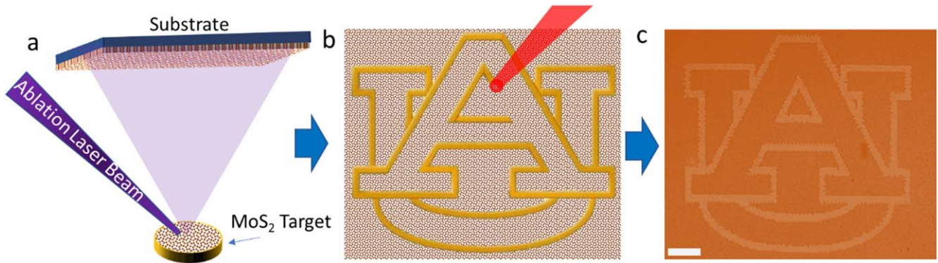
Figure 1. Schematic representations of the experimental design and process flow. Pulsed laser deposition (a) and laser writing/crystallization setups (b) were used for deposition of amorphous thin films and crystallization/writing of 2D materials, respectively. The optical image (c) shows a representative laser-crystallized MoS 2 pattern (Auburn University logo) on the fused silica substrate. The bright lines and dark background indicate the crystalline and amorphous regions, respectively. The scale bar is 200 \mu\text{m} .
